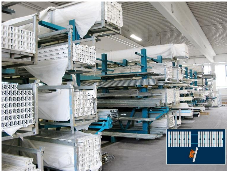
Image 2: With the crosswise HEGLA long-goods storage system, companies can store up to 50 percent more in an existing surface area. Movement to a gap brings the pallets into position for direct access.
